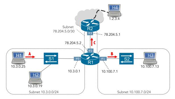
a) First, H1 sends an IP packet to H3. (Assume that this sends an ARP request, which happens successfully.) For the IP packet, write the source and destination addresses in both the L2 (Ethernet) and L3 (IP) header when it is crossing the link labeled A in the figure. For MAC addresses, you can use names based on the name of the host or router interface, eg. MAC\_H1 for H1, MAC\_IF1 for R1's IF1, etc.
