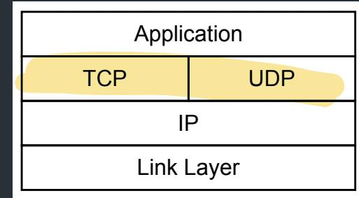
Creates a "pipe" to send/recv data to another endpoint, like a file descriptor
