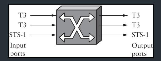
Switches must be able to, given a packet, determine the outgoing port
