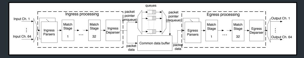
Current speeds reach 12.8Tbps (32x400Gbps or 256x50Gbps) on a single programmable switching chip
