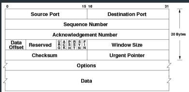
Computing the TCP checksum involves making a "pesudo-header" out of some IP and TCP header fields:
