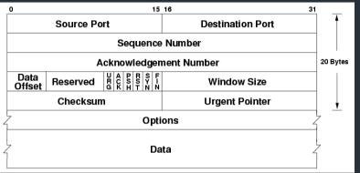
Computing the TCP checksum involves making a "pesudo-header" out of some IP and TCP header fields:
