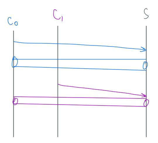
In TCP: each client gets its own connection--you can think of this as a unique "pipe" with which the server can communicate to each client independently.
